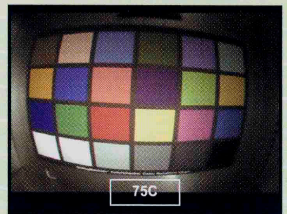
Low light image quality under high temp. @15 Lux
