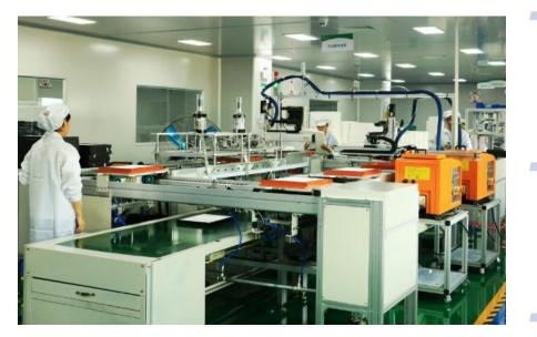
Integrated automated filter production line for edge sealing, injection molding, sealing treatment, and finished packaging
